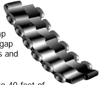
Wrap-It links are designed to make a hydrostatic seal of up to 20 psig and up to 40 feet of head. The Wrap-It links, in addition to its sealing properties, helps absorb vibrations, shock and sound waves. It also insulates the inner pipe from all other outer structures, including outer pipe sleeves, pipeline crossings, walls and tanks.
