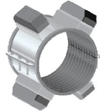
The runners shall be Glass Reinforced Polymer with ends of the runners beveled to facilitate installation over rough weld beads or the weld ends of misaligned or deformed casing pipe. The runners shall be attached to support structures (shell or risers) at appropriate positions to properly support the carrier pipe within the casing and to ease installation. They shall have a minimum length of 11.0 in. and a minimum width of 2.0 in.
