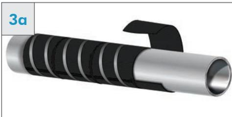
Cut to length for larger diameter pipelines or field joints by circumferentially wrapping cut sheets from bulk rolls.
