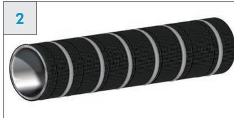
... spirally wrap from bulk rolls for larger diameter pipelines.
